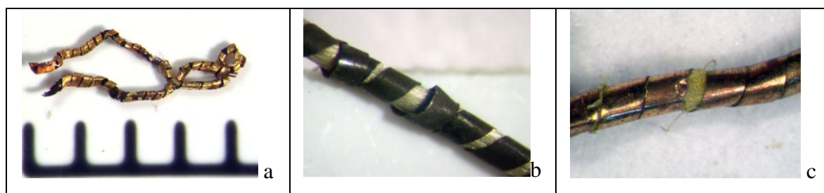
Fig. 2. OM images of file threads a) gold b) silver (tarnished) and c) copper/brass (a) scale 4mm and b,c ) mag. X40)
